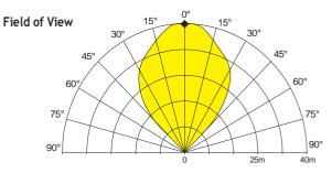
To meet the requirements of EN54:10 clause 5.4, where the ratio of the response points.  ${\bf Dmax:}\ {\bf Dmin}\ {\bf should}\ {\bf not}\ {\bf exceed}\ {\bf 1.41},\ {\bf the}\ {\bf horizontal}\ {\bf and}\ {\bf vertical}\ {\bf viewing}\ {\bf angles}\ {\bf max}\ {\bf should}$ not exceed ±30°.
