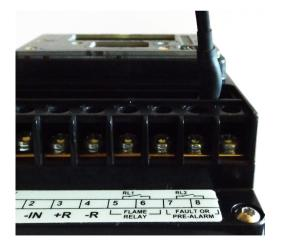
Connect the other end of the calibration cable to the USB-C socket on the top side of the TalentumTT<sup>2</sup>.
