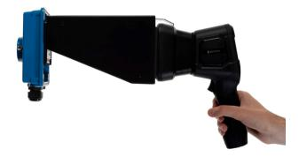
The following confirmation screen will be shown. Press the **Trigger** button to start calibration or the **Back** button to cancel Connections... ☑ Recalibrate Talentum WARNING: UV light! Attach shroud and serial cable to test Torch and Talenum. Confirm: Connected ! The Talentum TT<sup>2</sup> should connect to the Flame Detector in under five seconds. If this fails, see the "calibration errors" chapter on page 22.
