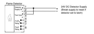
In self-test mode, the detector will check each of its sensors every fifteen minutes. If the test fails a Fault will be signalled.
