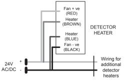
• The detector heater will draw an in-rush current on a cold-start (refer to specifications), which the power supply **MUST** be able to cope with.
